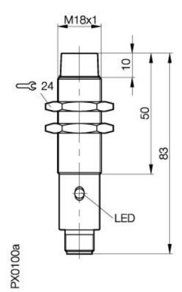
Inductive Sensors BES 516-360-S 4-H M18x1 x 83 normally-open Sn=8mm unshielded
